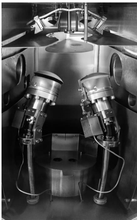
Figure 6.4. The interior of PVD process chamber in ML System laboratory with two magnetron sputtering guns: RF (left) and DC (right).
