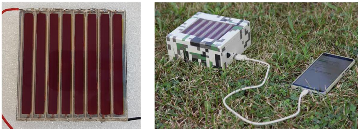
Figure 8.7. DSSC module, which was a part of solar charger prototype IMŁS0-2-W.
