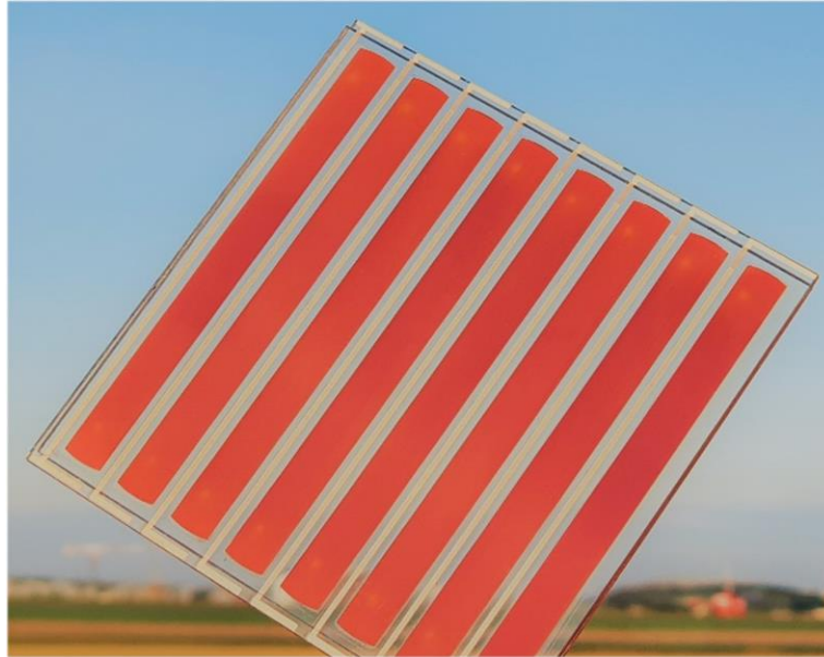
Figure 6.11. Photography of up-scaled module with 8 individual dye-sensitised solar cells.
