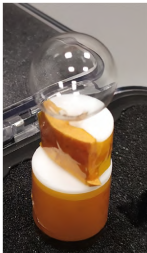
Figure 3.3: Atomic cell and a cell holder used in Kraków magnetometer. The cell is mounted with the Kapton tape. Between the tape and the stem, there is a piece of thermal insulation material.
