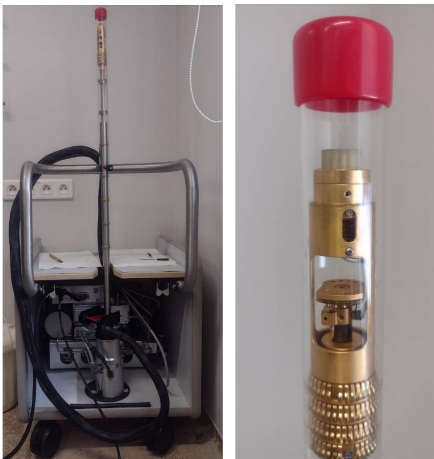
Figure 2.4.4 Left: The insert for the He-3 option. Right: the enlargement of a part, where the puck is mounted.
