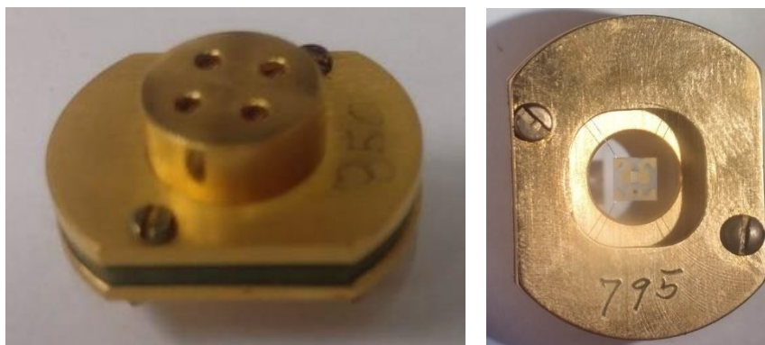
Figure 2.4.3 The puck for specific heat measurements with He-3. Left: the whole puck. Right: the interior of the puck. In the center, there is a sample platform fixed on the 4 wires.
