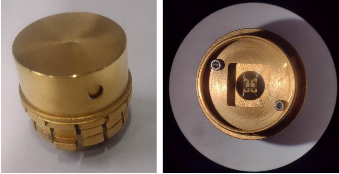
Figure 2.4.2 The puck for specific heat measurement with He-4. Left: the whole puck with a shield. Right: The interior of the puck. In the center, there is a sample platform fixed on the 8 wires. Under the platform, there are a thermometer and a heater mounted.
