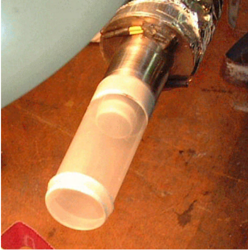
FIGURE 2.3: The LH 2 container used during the pp at 3.5 GeV experiment.
