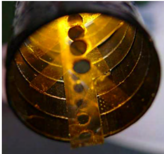
FIGURE 2.4: The segmented niobium target used for the p+Nb experiment. Niobium roundels are mounted by a tape inside a carbon tube.
