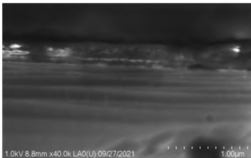
Figure 4.9. SEM image of a cross-section of a polished sample. Detection of backscattered electrons, magnification x40k
