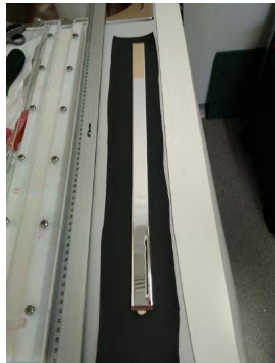
(b) the second wrapping is done by wrapped in ESR
