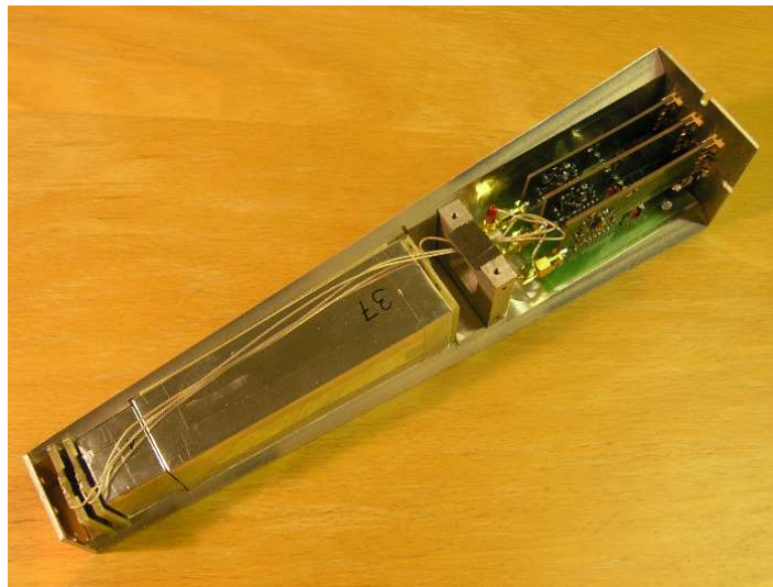
Figure 5.2: Single KRATTA module content: two CsI crystals wrapped in a foil and three Si photodiodes connected to preamplifiers.
