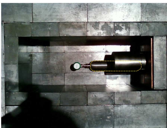
Figure 3.5: The transport bottle (dashed yellow line) placed under the germanium detector. View from the top into the lead shielding used for screening.
