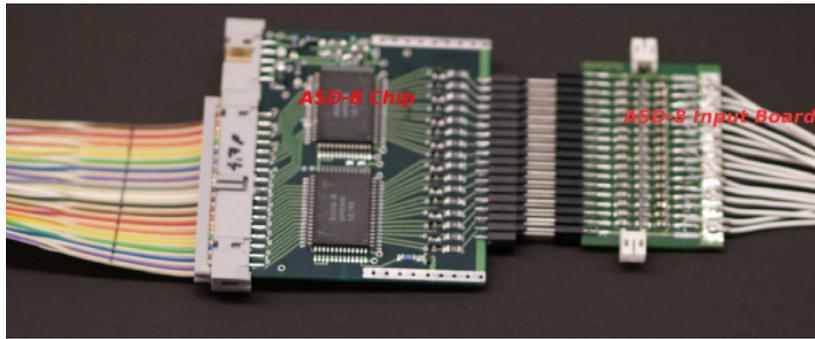
Figure 5.7: (Left) Front-end board with two ASD-8 chips. (Right) the input board to match the amplitude of the signals from the preamplifier and shape them for the ASD-8 chip [19].
