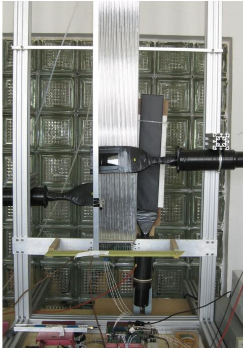
Figure 4.7: Prototype straw tube tracker developed at the Jagiellonian University for the PANDA Forward Tracker. The scintillator detectors are used to provide timing measurements.
