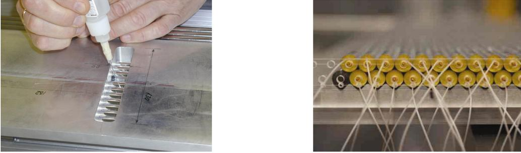
Figure 1.9: (Left) gluing of straw tubes in a double layer on a reference table, (Right) a straw tube double layer. Two layers of straws in a double layer are shifted with respect to each other by half of the distance between the straws in order to resolve the “left-right” ambiguity of the track position with respect to the anode wires [10].
