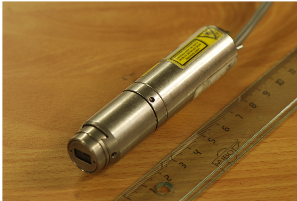
Figure 2.2.1: Lasers used for illumination of pellets
