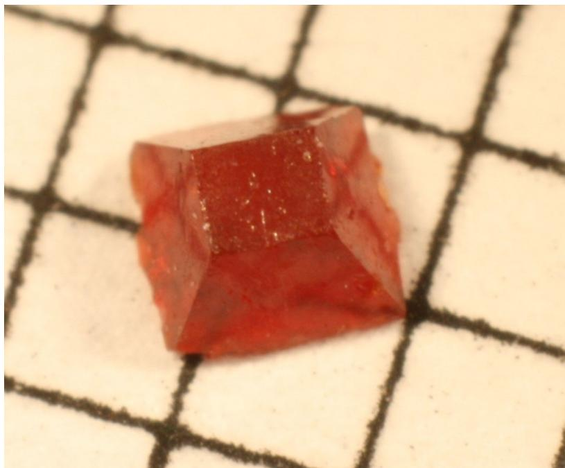
Figure 3.6: Photography of the top-cut pyramidal-shaped single crystal sample of  $Mn_2^{II} - Nb^{IV}$  used for magnetic measurements. The size of the grid on which the crystal was photographed is 1mm.
