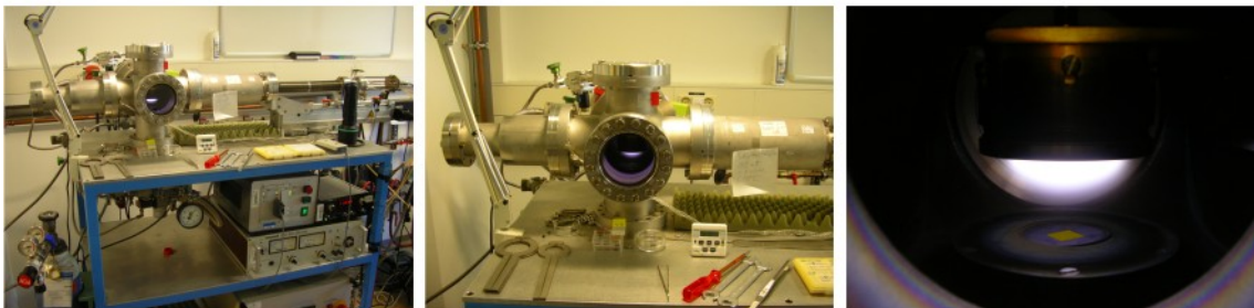
Pictures of the HPS deposition chamber designed and built by Dr. Ulrich Poppe, under operation in Peter Grünberg Institute in Forschungszentrum Jülich (Germany).
